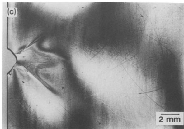
Figure 4 The yield zone of 6.54 mm thick PC near position 3 viewed in the polarizing optical microscope. (a) The full thickness with polished surfaces, (b) with 1.5 mm of the thickness removed from each side, and (c) with 3.0 mm of the thickness removed from each side.
