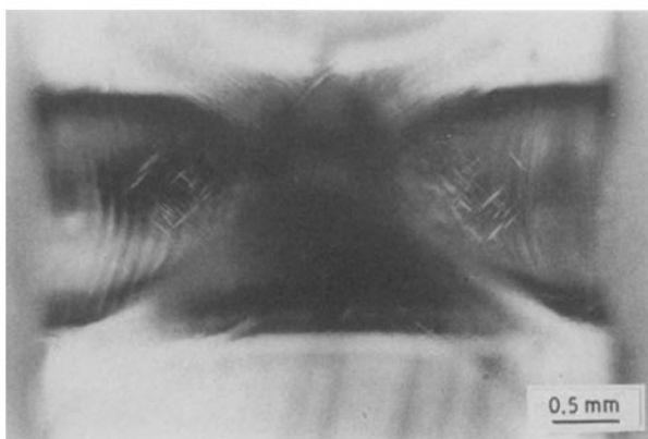
Figure 10 Polarized light micrograph of the yield zone of 4.70 mm thick PC at position 4 sectioned at the position of the arrows in Fig. 9d and viewed in the yz plane.
